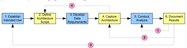
The first common type of iteration (1) is where having generated the architecture there are periodic analysis / update cycles without any major refresh of the architecture itself. This approach may apply for example to the development and detailing of a number of capability options within the Sponsor's processes of finalising the Equipment Programme.
